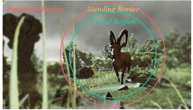
Fig. 11: Implementation of our gaze-contingent rendering. The inner circle denotes the foveal region, which is rendered with high fidelity; the blending border refers to the transitional region; and the outer region is the peripheral region rendered with low quality.
