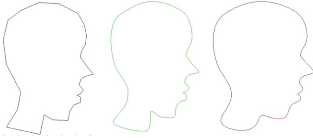
Fig. 8. An example of differential space subdivision for curves. From left to right are the control polygon, its four-point subdivision curve, and its differential space four-point subdivision curve.
