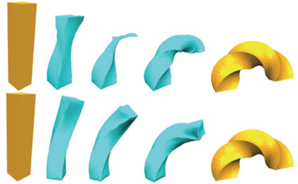
Figure 4: Comparison of linear interpolation (top) and our approach (bottom) between two severely deformed shapes (yellow). The interpolated shapes (cyan) are shown for interpolation weights of w_1 = 0.25 , w_1 = 0.5 , w_1 = 0.75 .
