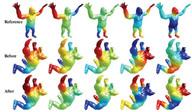
Figure 2: The eigenfunctions of a deformed armadillo are registered with respect to the eigenfunctions of a gorilla. After the registration, the eigenfunctions between the shapes are consistent. Hot and cold colours represent positive and negative values, respectively.
