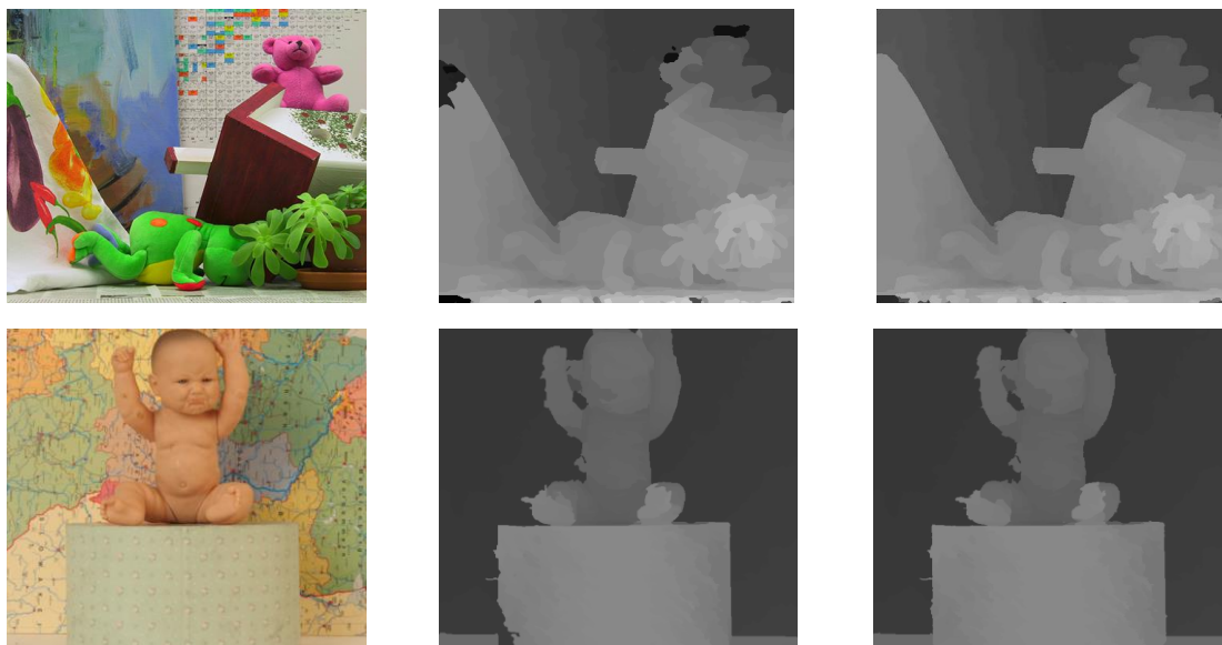
Figure 7 The disparity results of Teddy and Baby1 stereo pairs. From left to right: Original left images; disparity results without segmentation-aided checking; disparity results with segmentation-aided checking.
